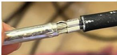
Correct terminal crimping:
